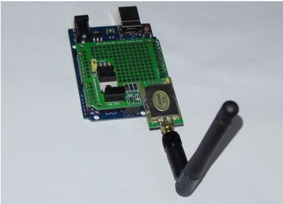
Shown above configured with high power nRF24L01+ module using SW SPI, Vin voltage regulator input source selected.
