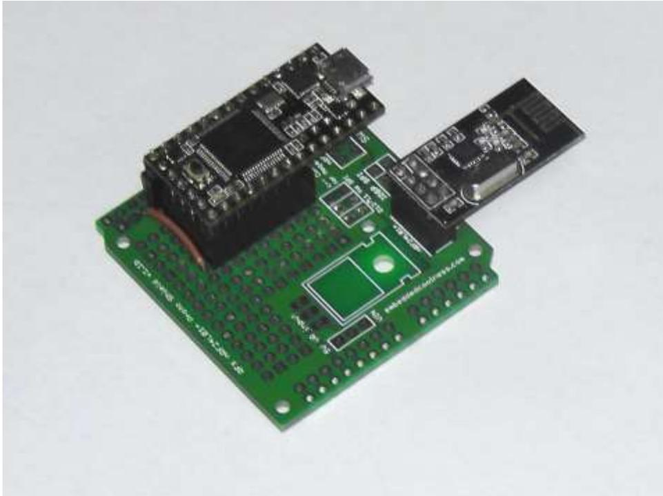
Although not designed primarily as a Teensy 3.x “carrier board”, the shield can be adapted to compactly host a Teensy 3.x dev board in a fairly straightforward way, described below.
